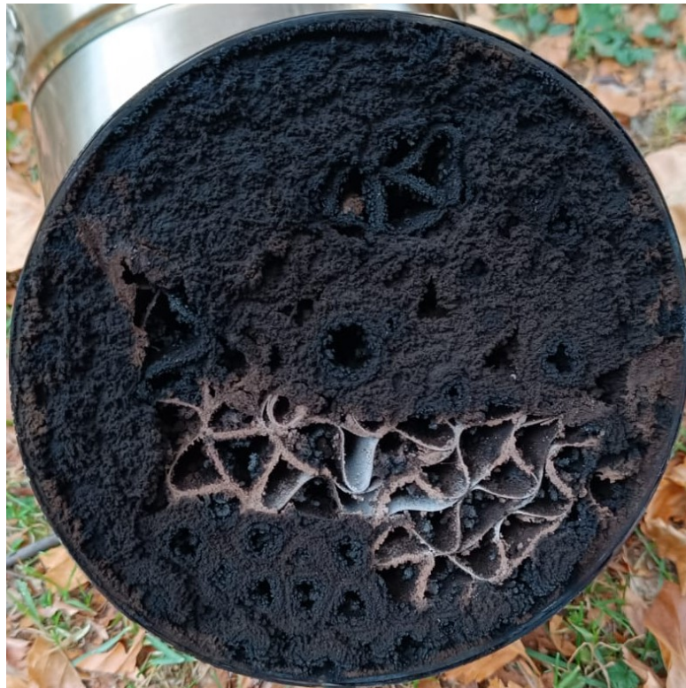
An example of creosote plugging on the face of the catalytic combustor
